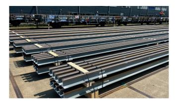
2. Since we had no information about the handling or unloading procedures at the port of Hong Kong, we had to prepare the bundles to accommodate both crane and dual forklift handling. The number of rails per bundle and the total number of bundles had to be adjusted to ensure optimal utilization for truck transportation to the port, as well as for maximum efficiency on Mafi trailers.
