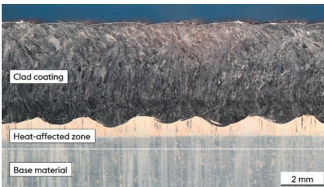
Cross-section view of a laser clad coating
