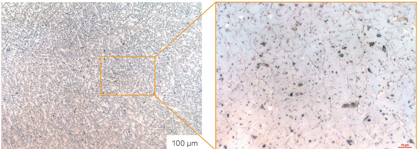
Structure of a laser-deposited Fe-Cr-Mo coating
