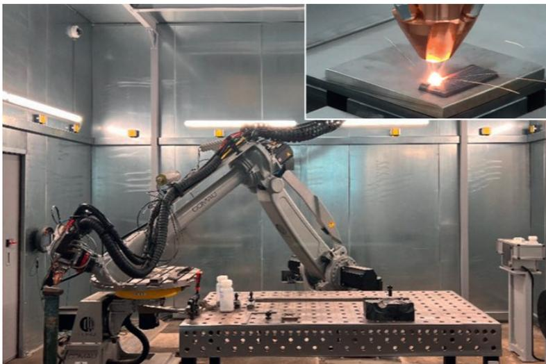
Robotic 6 – Axis CNC laser system
