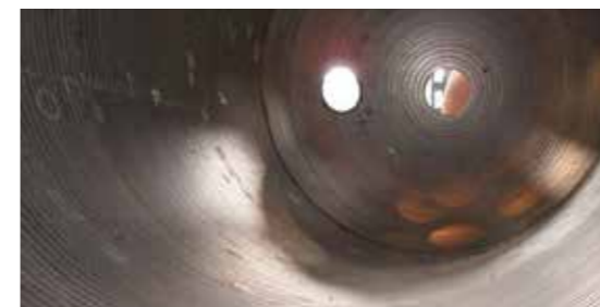
Pressure Vessel (Stainless steel alloy 347) SOUDOTAPE 24.12 LNb + RECORD EST 136
