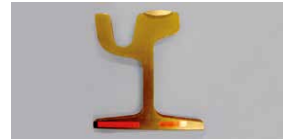
Rails hardfacing (austenitic stainless steel 307L) SOUDOTAPE 309L + RECORD EST 307
