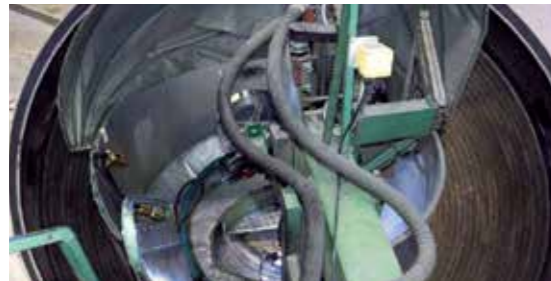
Reactor Vessel SOUDOTAPE 309L Q5 + RECORD 6/74 Q5
