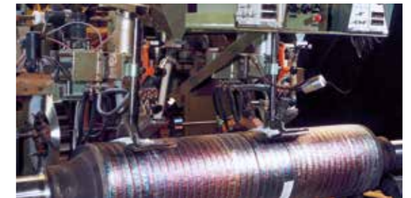
Steelworks - Continuous Casting Rollers (13 6 2 L) SOUDOTAPE 430 L + RECORD RT 168
