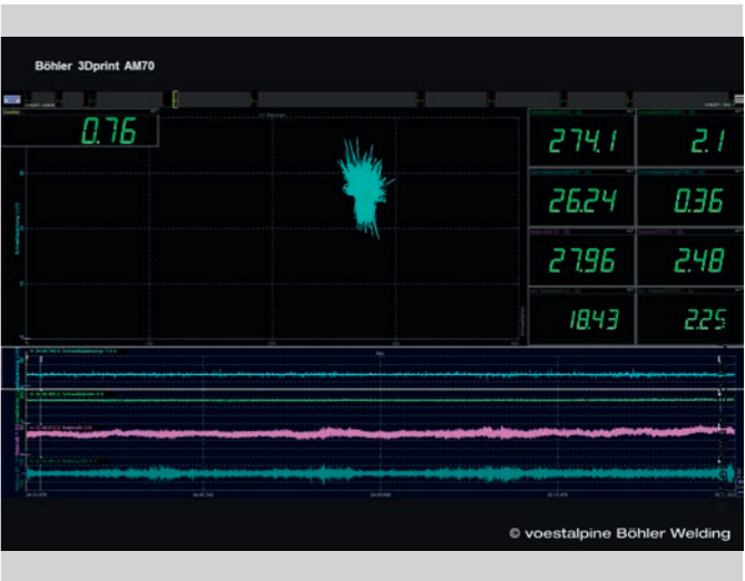
U[V]/I[A] integral plot over time (blue star in the middle) of stable process which shows only minor deviations
