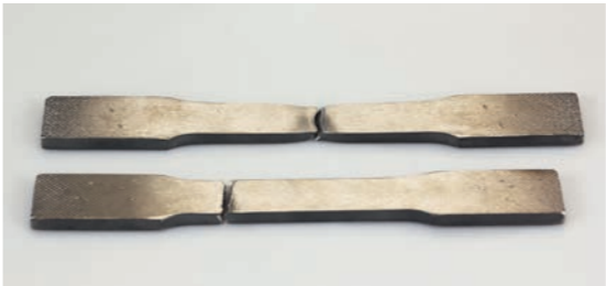
Printed coupon and destructive tests on precipitation hardening martensitic stainless steel 3Dprint AM 17-4 PH deposit
