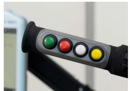
5 Wireless Control buttons: Green – add points along the welding path Red – welding on and off mode White – active robot-free drive mode Yellow – linear movements
