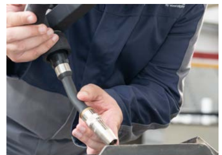
Simply move the robotic arm to the work piece and start teaching.
