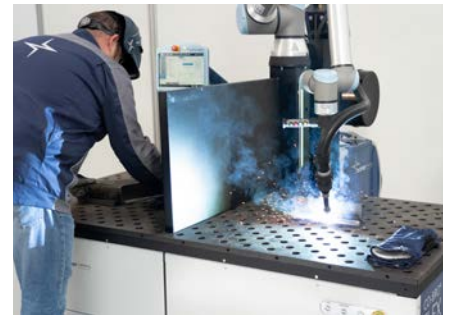
3 Integrated table divider – simultaneous welding and positioning of the next workpiece.
