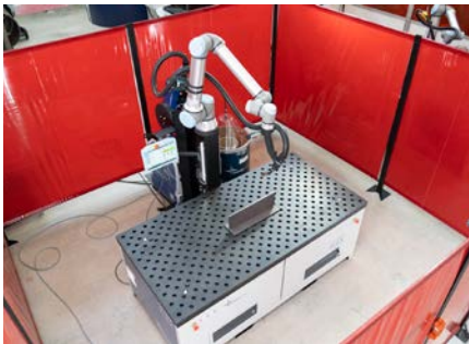
Once the peripheral protection is closed, the machine turns into a full robotic station.
