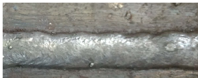
WEARcore XD 62-O welded with Current of 350 AMP
