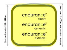
endurance tubes include the curvature tolerance in the dimensional tolerance
