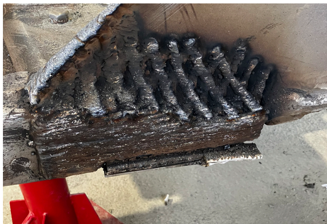
Figure 4 A.) UTP ROBOTIC CHROMELESS 600 weld overlay welded in PF position with oscillated beads and using pulse technique
