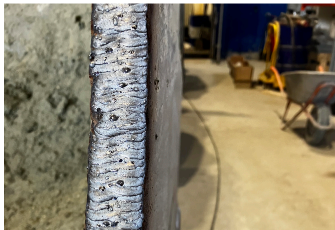
Figure 4 B.) Buffer layer applied using the all-positional rutile Böhler FOXcore 309L-T1 welding wire
