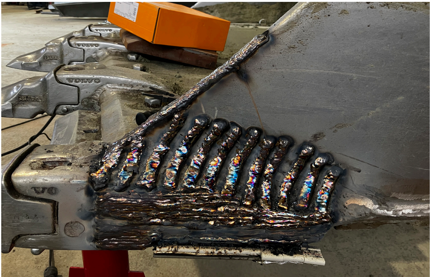
Figure 3 B.) - Buffer layer applied using the all-positional rutile Böhler FOXcore 309L-T1 welding wire.
