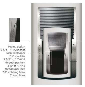
Casing design 5 – 7 inches 10 % seal taper 15° shoulder 5 threads per inch 10° stabbing flank 3° load flank
