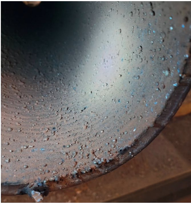
Figure 3. Actual view of the ID of one of the field tested long radius elbows hardfaced using WEARcore XD67/1-O after 15,000 tons throughput. Note the spiral weld beads are still visible which indicates a very low material loss.
