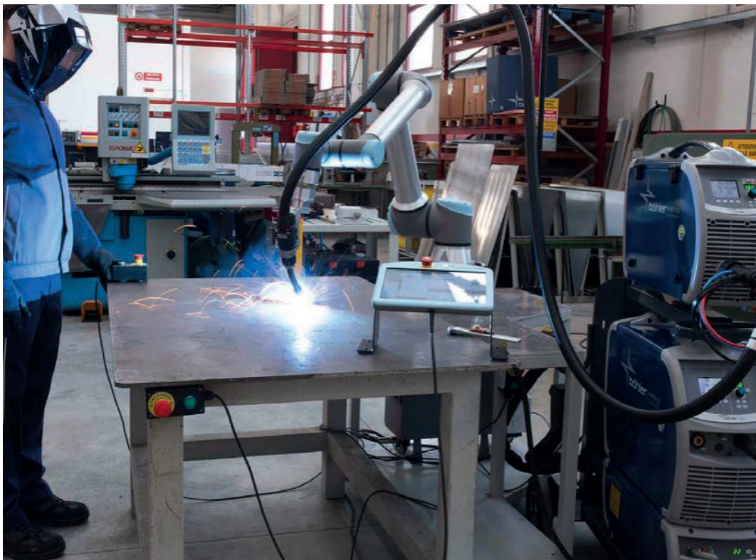
A collaborative robotic welding installation
