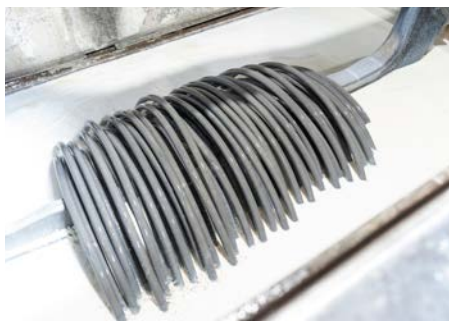
Coating of coils
