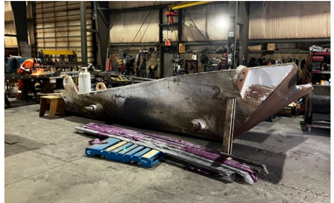
Figure 4: Molten nickel chute, side view.
