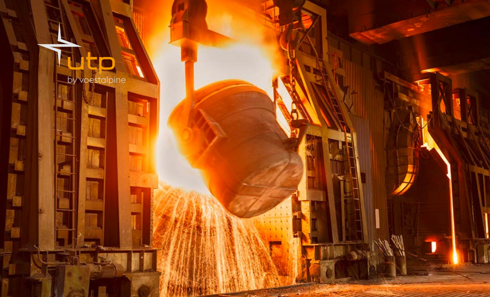
Figure 1: Pouring ladle in action. (Source: https://www.eastcarb.com/ladle-furnace/ )
