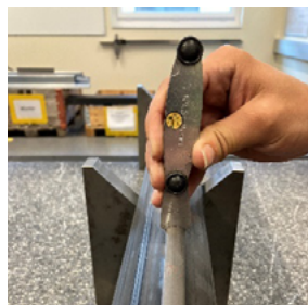
Measurement of the radius using a radius gauge Result: R_a
