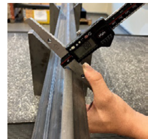
Measurement of the radius contour using a caliper Result: C_1, C_2
