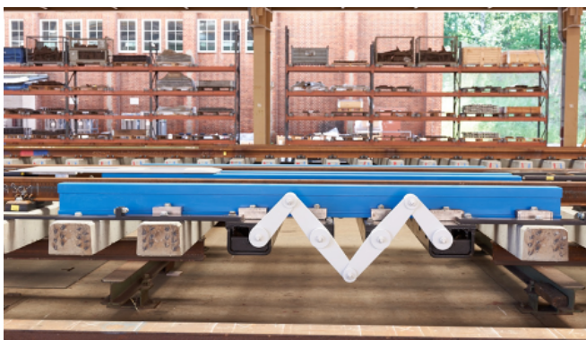
auxiliary bridge with scissor system
