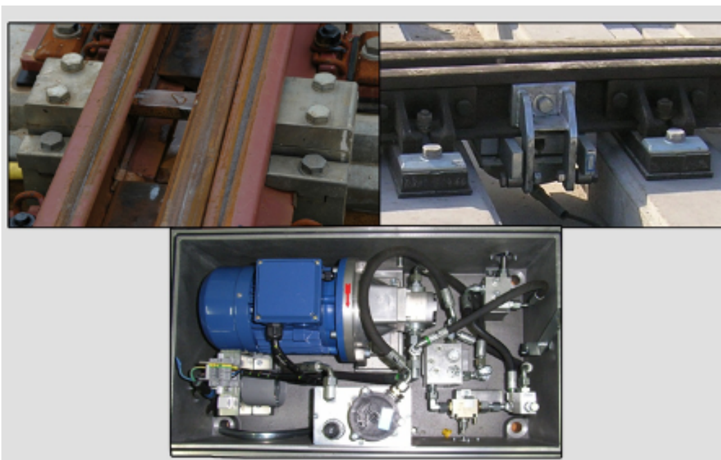
Assembled holding down device and opened drive unit
