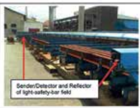
Figure 4.9b: ...and in horizontal position additionally for surveillance that nobody is staying within an area – see example automatic conveyor line of sawing-drilling unit. There are different classes of light/lasers (different range in covered distance and number of rays per meter (for different stages of safety like "finger-proof", "arm-proof" or "body-proof")); outdoor and especially above 30m distance light bars will be problematic due to false signals (rain/fog/birds...)
