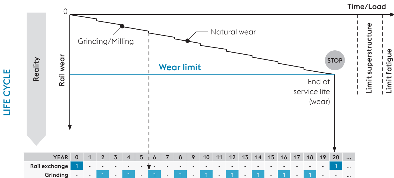
Figure 3: Schematic example for the life cycle of a rail in a curve with specific annual traffic load and radius
