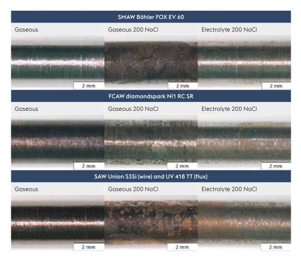
It is possible to observe no fracture on all the all weld metal specimens in both dry and wet conditions.
