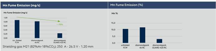
The fume emission data were generated under laboratory conditions as described in EN ISO 15011.
